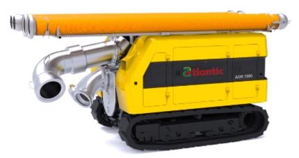
The ADR 1580 is Atlantic's Drainage and Water Supply Robot designed for flood-prone areas and confined spaces like underground parking lots, basements, metro and subway stations, underpasses, caverns, and stormwater tunnels. It offers quick mobility, fast operation, long runtime, and reliable safety features. This dewatering robot is an efficient alternative to large emergency response vehicles and is ideal for rainwater extraction from tight spaces and search-and-rescue operations.
